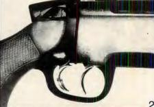
4. Military-type three-position safety. In the rear position, everything locks; in the middle position, rifle is on safe, but bolt can be operated; in the forward position, it's ready to fire.
